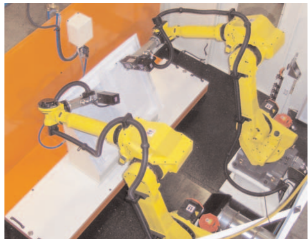
An inside view of the RoboTrim RT-1202 router trimming system shows the two floor-mounted AccuTrim R-110 robots.
