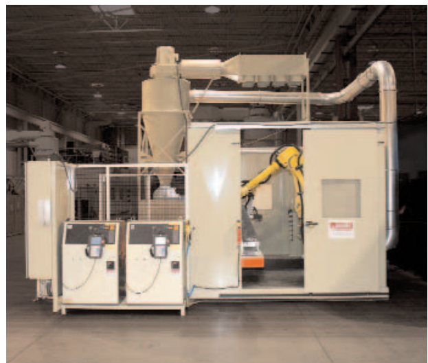
This side view of the RoboTrim RT-1202 router trimming system shows the two FANUC R-30iC robot controllers and a glimpse of the AccuTrim R-110 robots through the sliding side access door.
